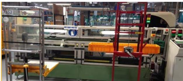
Examples of ergonomics via adjustable lifts for parts containers and machine safeguarding (Vitré, France)
