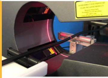
Integrated extrusion control allows 3D profile control and surface defect detection
