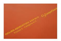
The standard DIN VDE 0680 Part 1 was superseded by the European Standard IEC 61112 in March 2010. The change to a European standard also increased the requirements applying to insulating blankets, which the previous EPDM (ethylene-propylene diene monomer) grade A-KX 50-10 was no longer able to fulfil.
