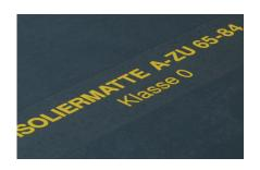
The standard DIN VDE 0680 Part 1 has now been superseded by the European Standard DIN EN 61111. This change to a European standard also increased the requirements applicable to insulating mats, which can no longer be fulfilled by the tried and tested natural rubber grade A-BY 60-84.
